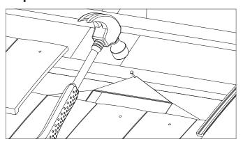
The top and side underlay triangular shapes should be folded outward and underneath the ventilator. The top triangle should be pulled tightly and tacked to the batten above.
