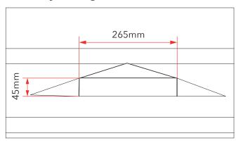
It is important that the cut forms a snug fit to the ventilator to deflect and prevent water and debris penetration through the underlay.
