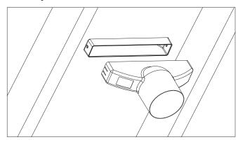
The ventilator must be accessed from the underside. Fit the Pipe Adaptor (code: HD DPCA) over the spigot on the underside of the ventilator ensuring the adaptor clips onto the spigot securely
