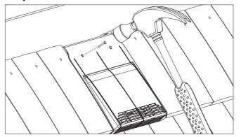
Position the ventilator with the spigot through the underlay cut and nail the ventilator to the batten through the holes in the top flange.
