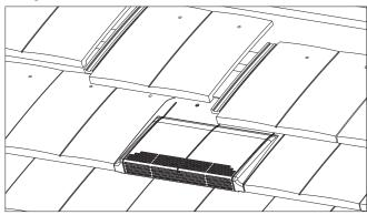
With the ventilator in position, tiling can be completed, leaving a discreet flush fitting installation.
