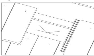
Once the position of the ventilator has been determined, mark and cut the underlay in a V-shape to the size shown below.
